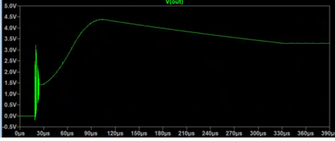
Fig. 6. Voltage peak with no Zener diode and with the soft-start circuit
