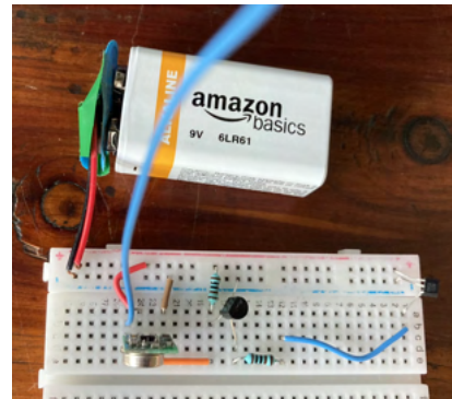
Fig. 26. Implementation of transmitter with wind sensor
